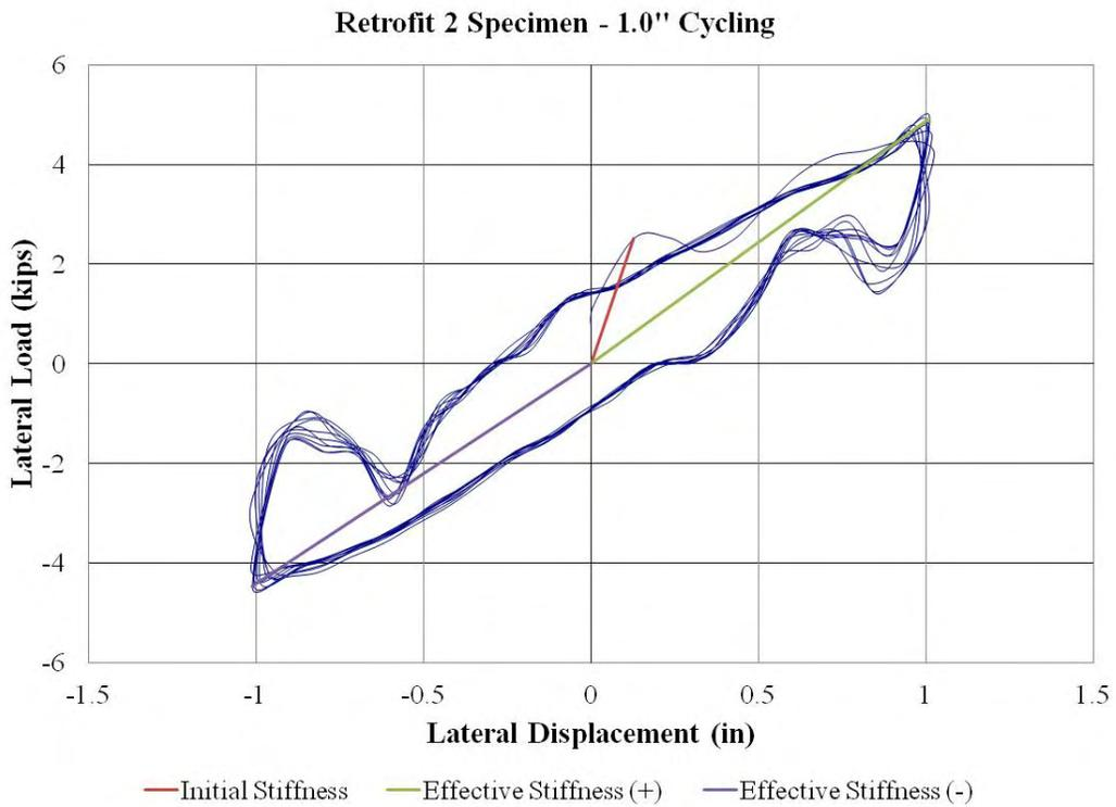
**Figure 81: Retrofit 2 Specimen – 1.0” Cycling**
