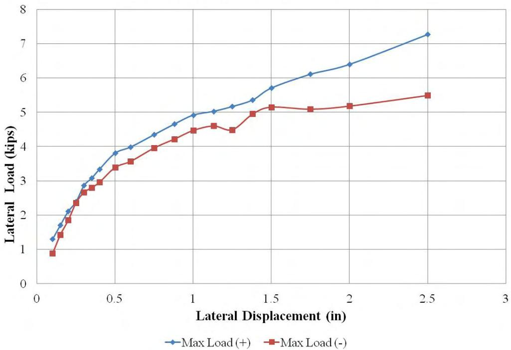
**Figure 50: Retrofit 2 Specimen Maximum Lateral Load**
