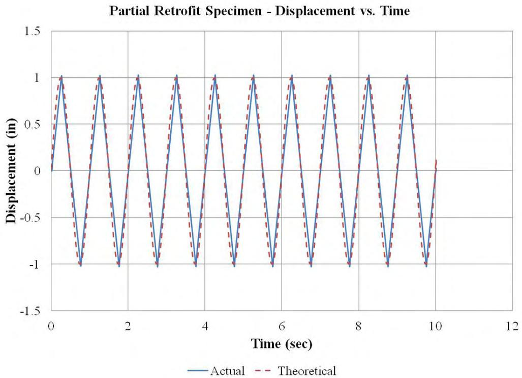
**Figure 24: Partial Retrofit Specimen - Displacement vs. Time**
