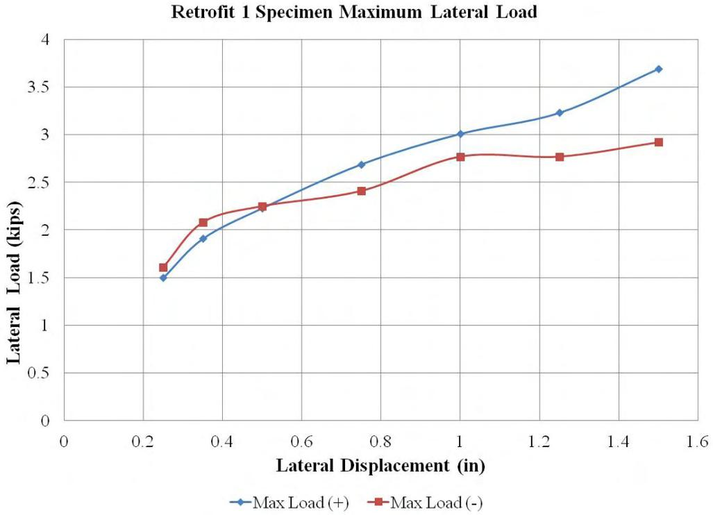
**Figure 43: Retrofit 1 Specimen Maximum Lateral Load**
