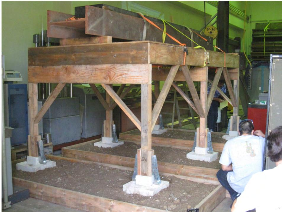
Figure 5: Partial Retrofit Specimen
