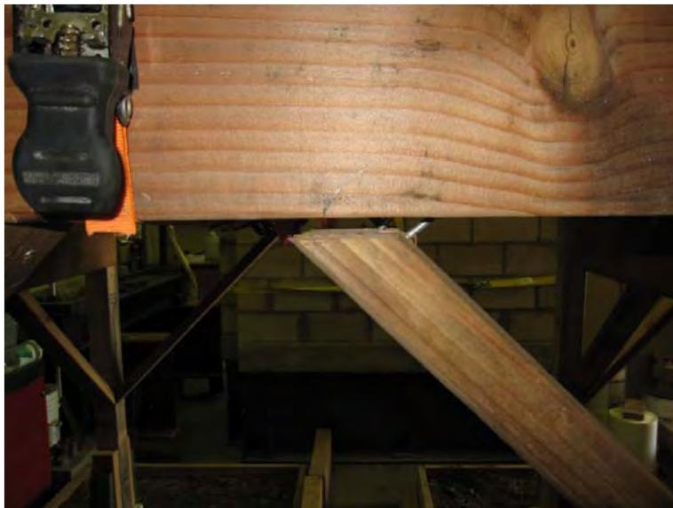
**Figure 38: Partial Retrofit Specimen Nail Pullout**
