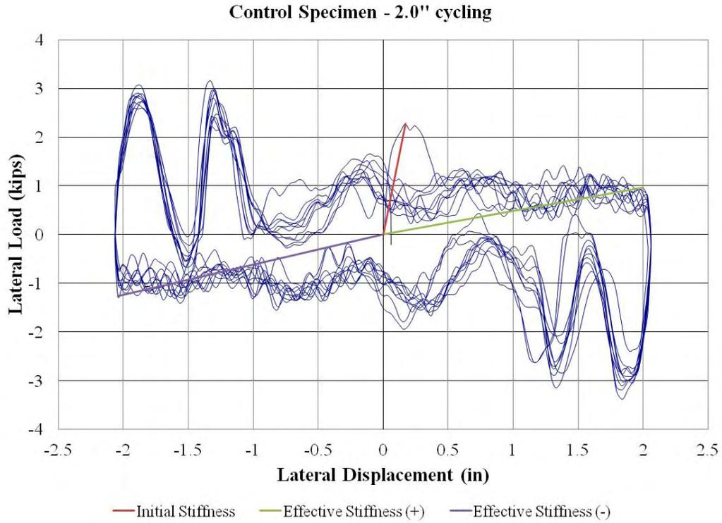
**Figure 28: Control Specimen - 2.0" Cycling**
