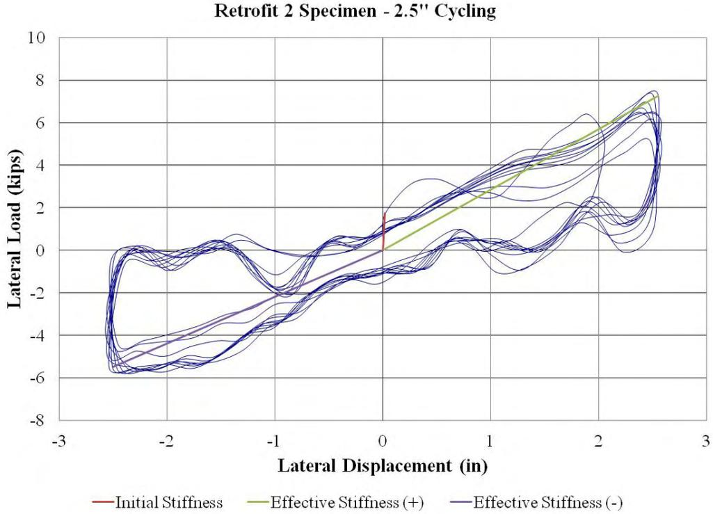
**Figure 48: Retrofit 2 Specimen – 2.5” Cycling**
