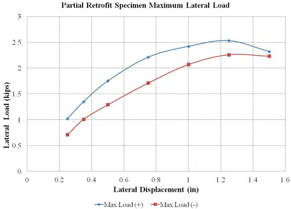
**Figure 37: Partial Retrofit Specimen Maximum Lateral Load**
