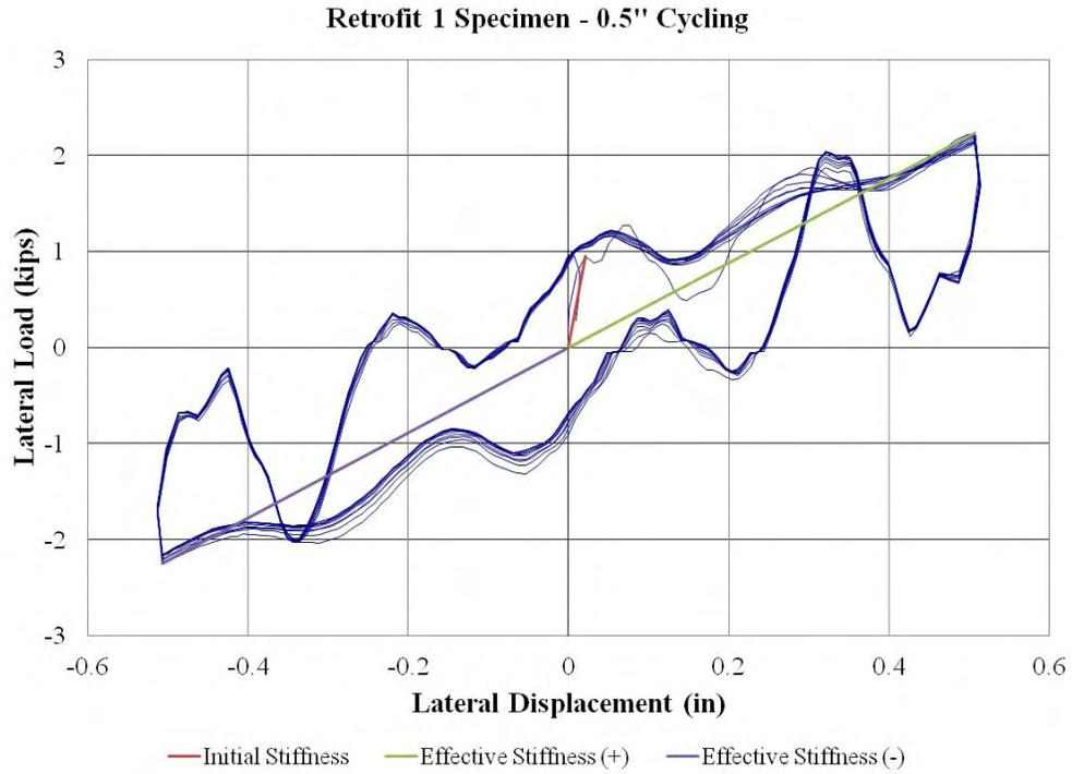
**Figure 40: Retrofit 1 Specimen – 0.5" Cycling**
