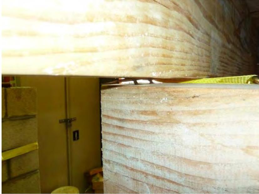
**Figure 39: 4x10 Perimeter Beam to 4x10 Girder Toe-nail Pull Out**
