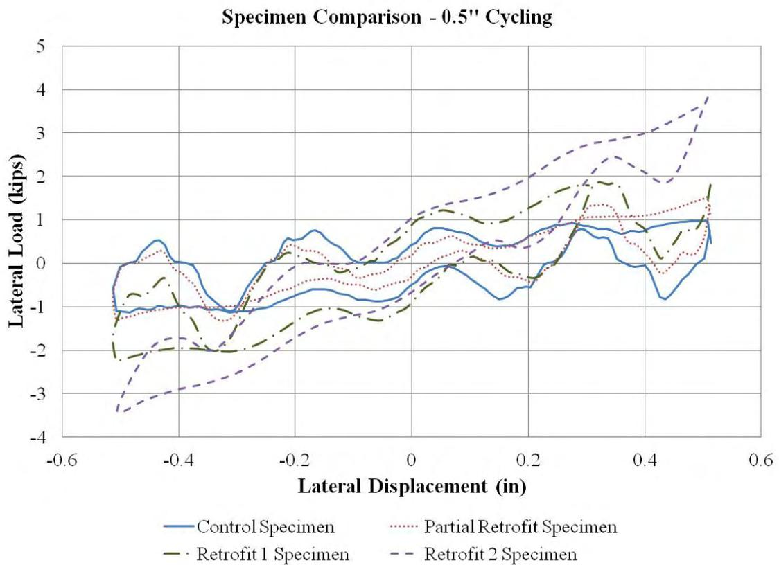
**Figure 52: Specimen Comparison – 0.5" Cycling**
