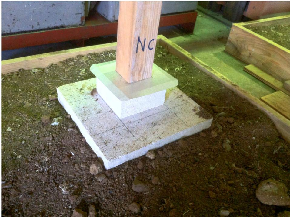
**Figure 2: Typical Un-Retrofitted Tofu Block Foundation**
