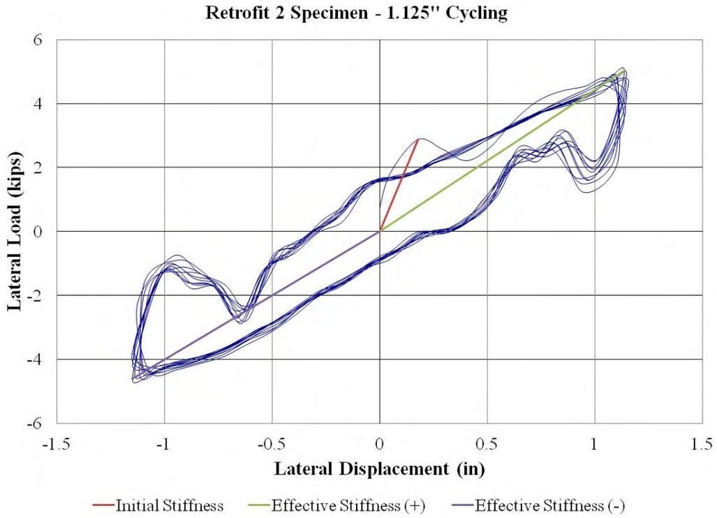
**Figure 82: Retrofit 2 Specimen – 1.125" Cycling**
