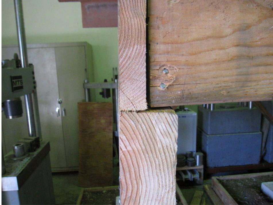
**Figure 46: 4x10 Perimeter Beam to 4x10 Girder Nail Pullout**
