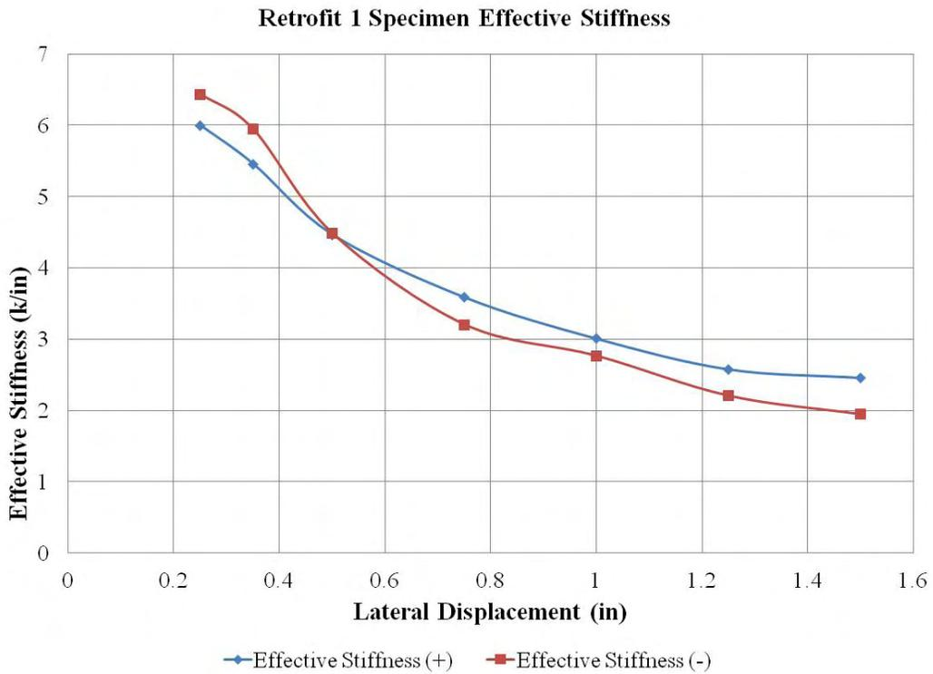
Figure 42: Retrofit 1 Specimen Effective Stiffness
