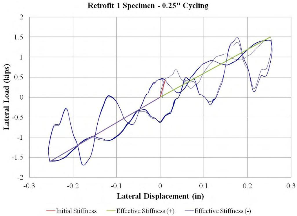
**Figure 66: Retrofit 1 Specimen – 0.25” Cycling**
