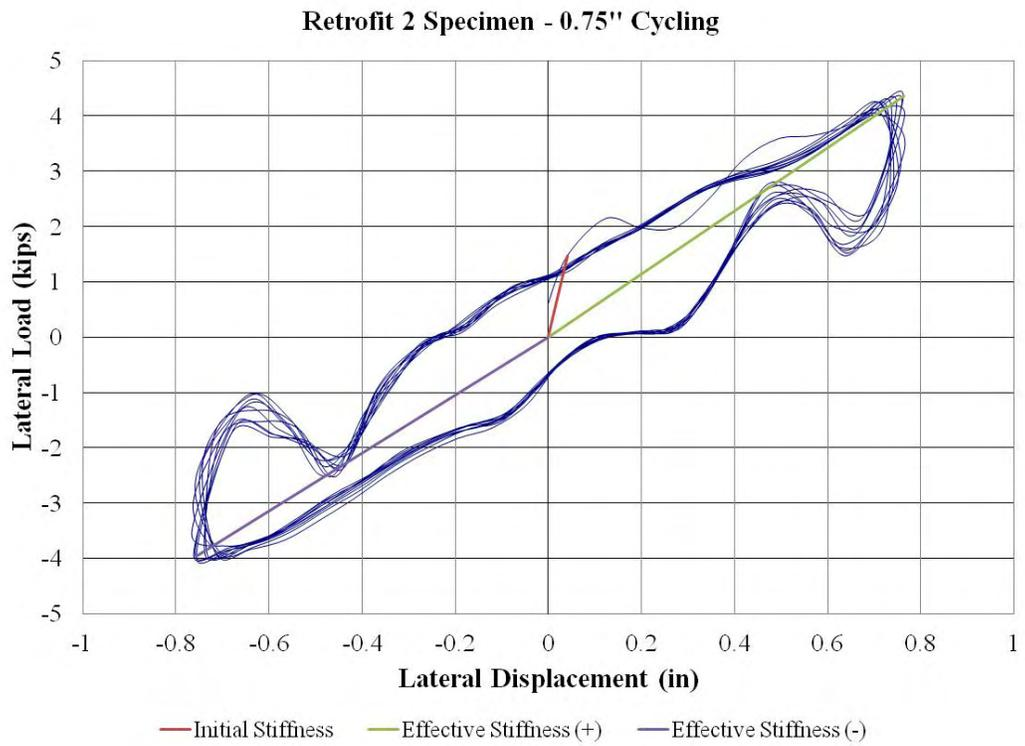
**Figure 79: Retrofit 2 Specimen – 0.75" Cycling**
