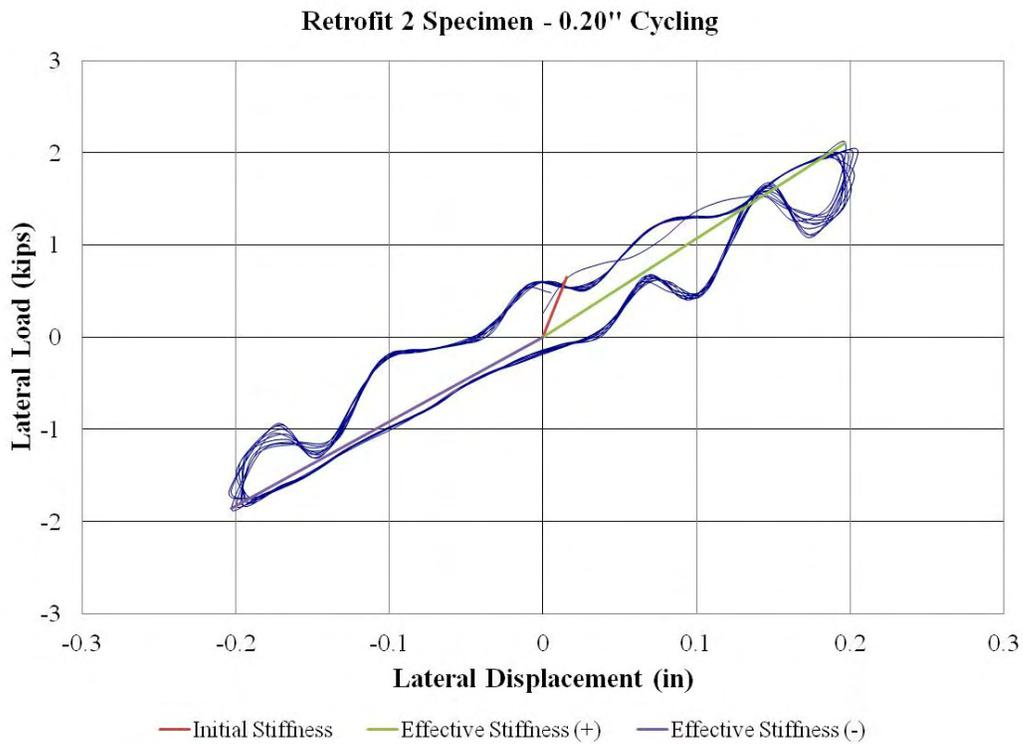
**Figure 73: Retrofit 2 Specimen – 0.2” Cycling**
