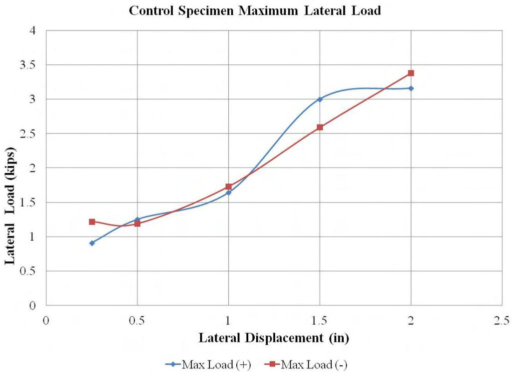
**Figure 30: Control Specimen Maximum Lateral Load**
