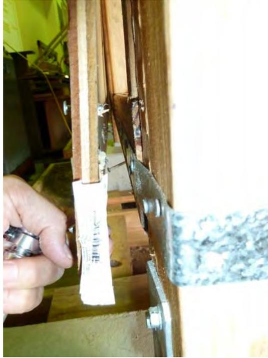
**Figure 51: Plywood Shearwall Edge Nailing Shear Failure**
