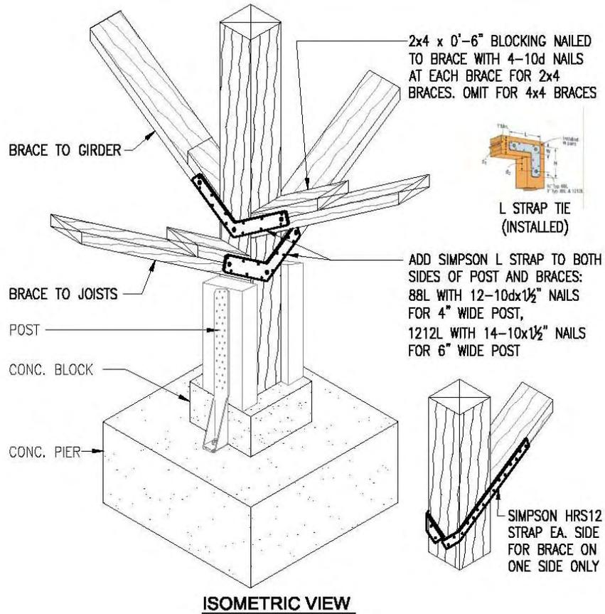
**Figure 10: Simpson 88L Strap installation**
