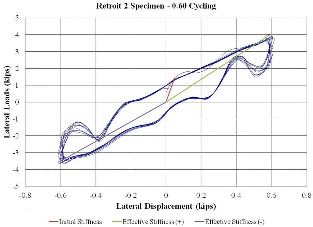
**Figure 78: Retrofit 2 Specimen – 0.60" Cycling**
