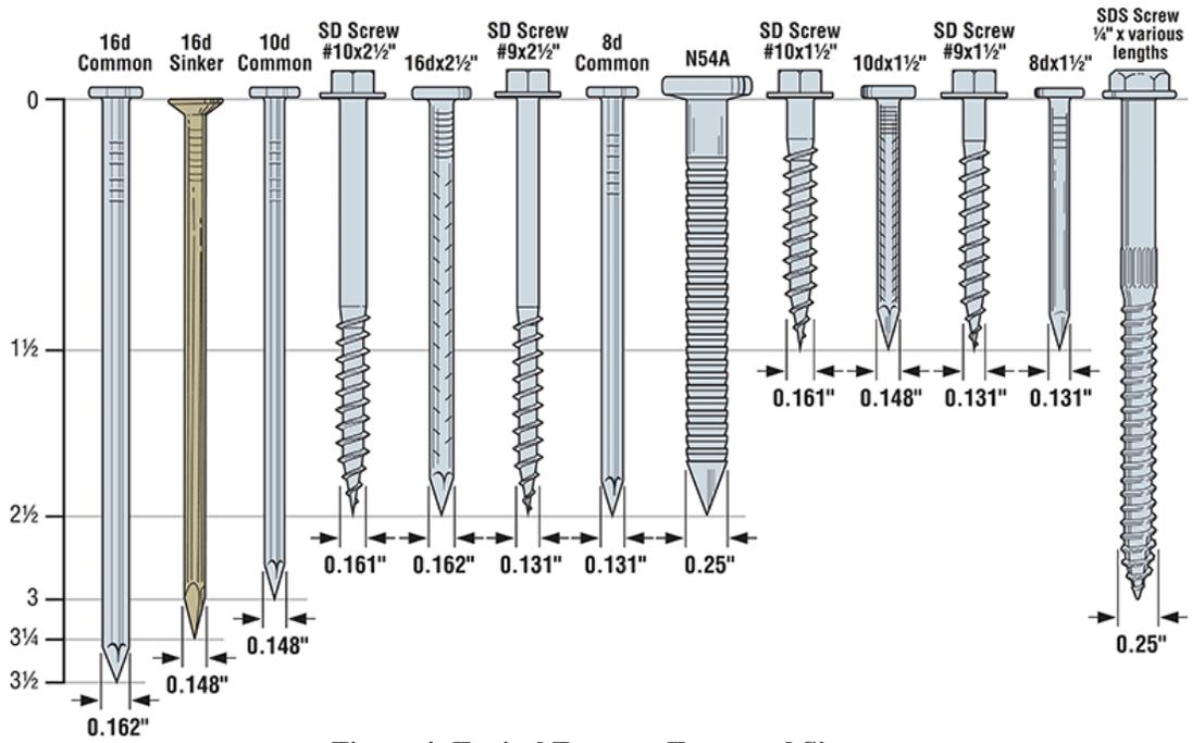
Figure 4: Typical Fastener Types and Sizes
