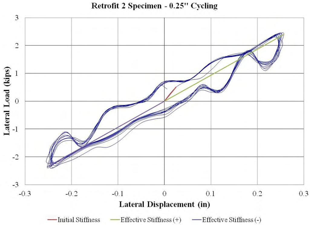
**Figure 74: Retrofit 2 Specimen – 0.25" Cycling**
