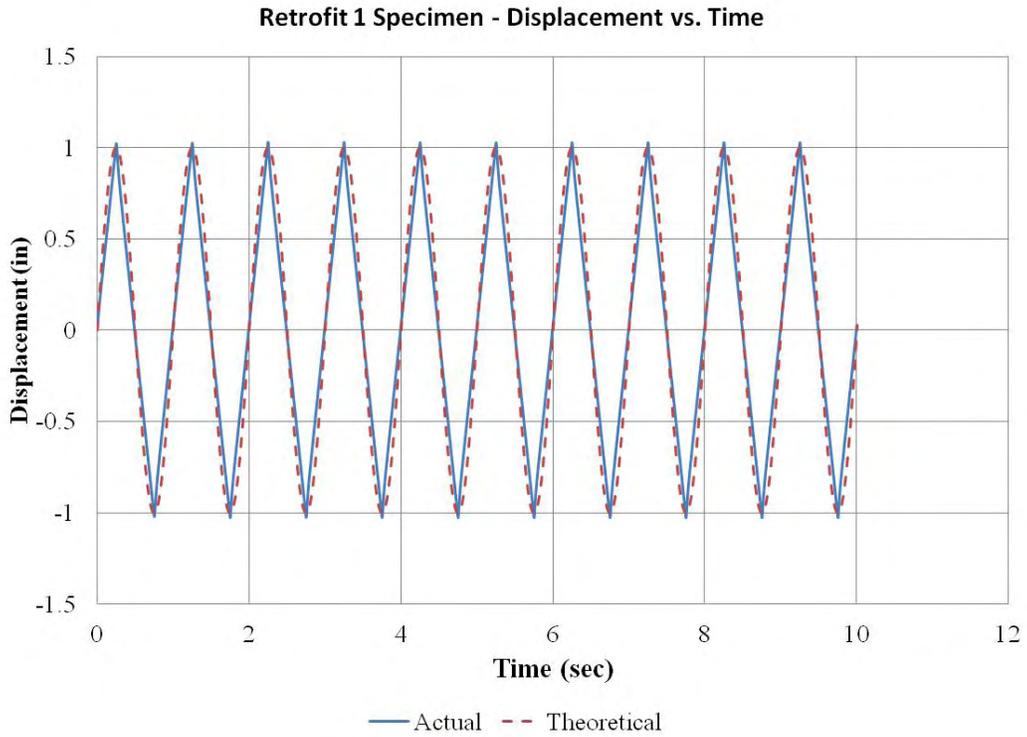
**Figure 25: Retrofit 1 Specimen - Displacement vs. Time**
