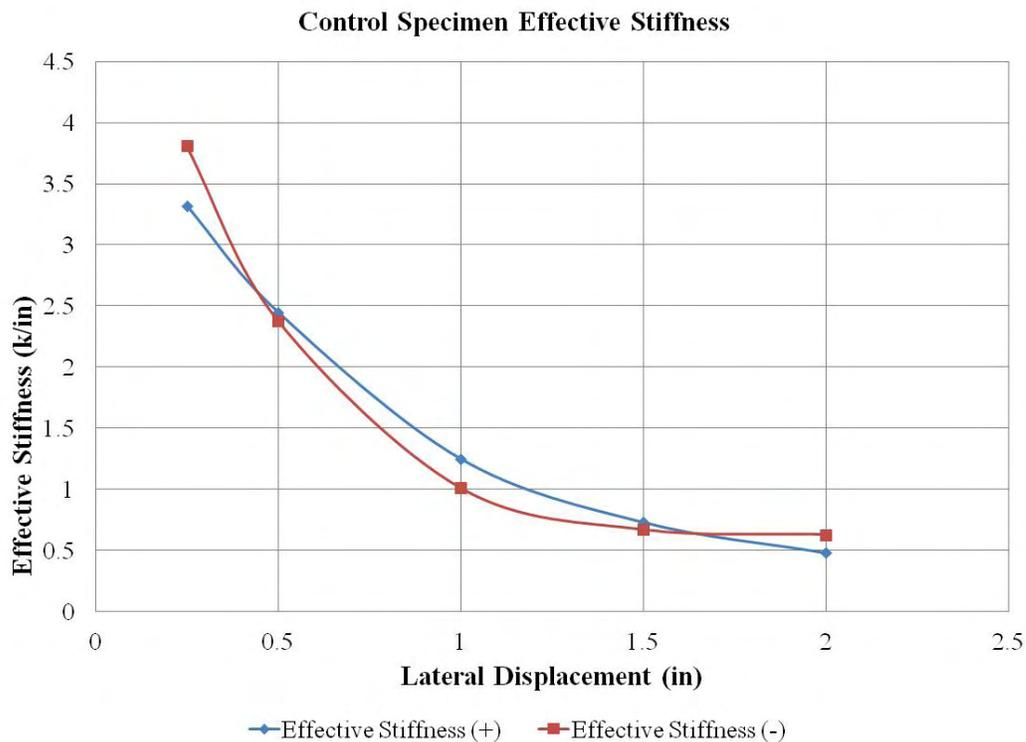
Figure 29 shows the decay of the effective stiffness of the specimen as the lateral displacement is increased. Figure 30 shows the maximum lateral load resisted by the foundation system during each set of 10cycles at increasing displacements.
