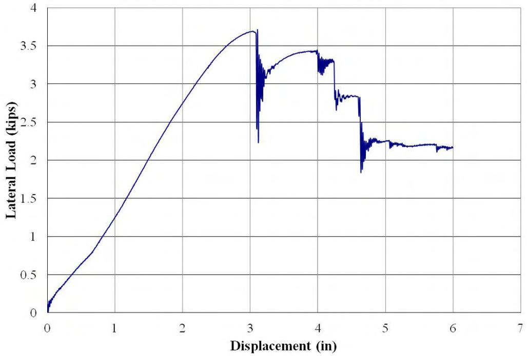
**Figure 44: Retrofit 1 Specimen Monotonic Pushover Test**
