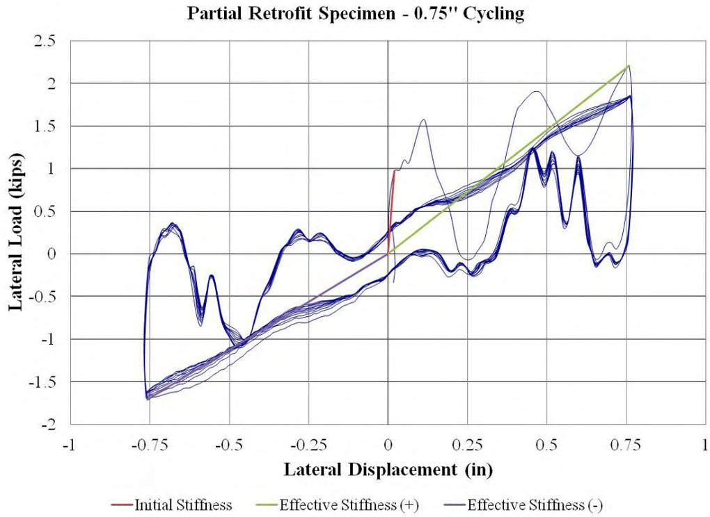
**Figure 64: Partial Retrofit Specimen – 0.75” Cycling**
