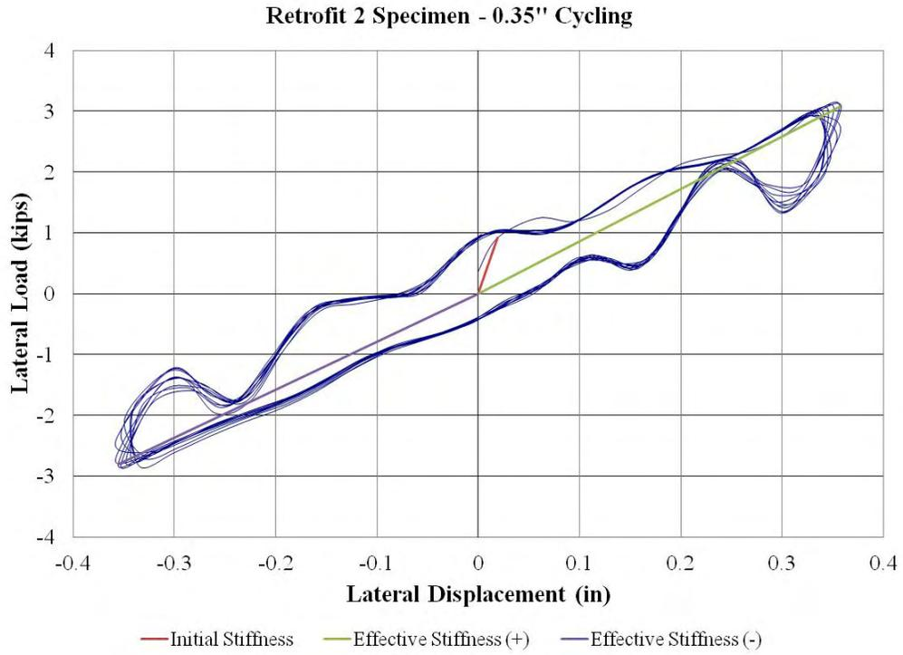
**Figure 47: Retrofit 2 Specimen – 0.35” Cycling**
