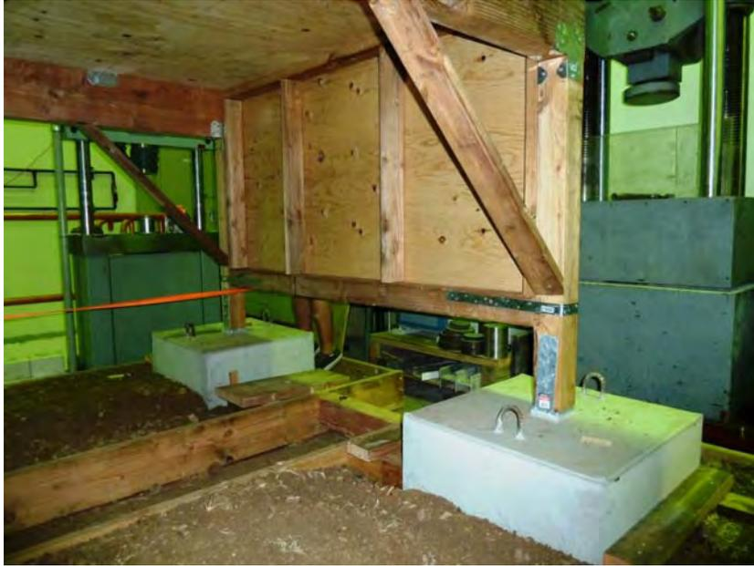
**Figure 21: Retrofit 2 Specimen Plywood Shearwall and Plywood Sub Diaphragm**
