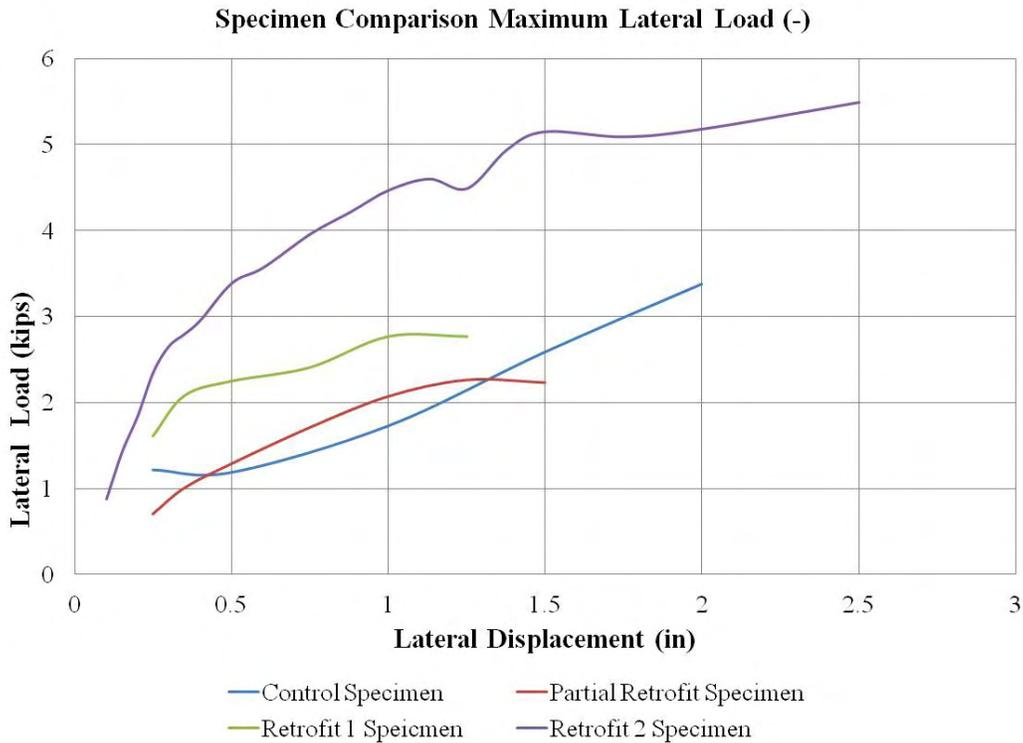
Figure 57: Specimen Comparison Maximum Lateral Load (-)
