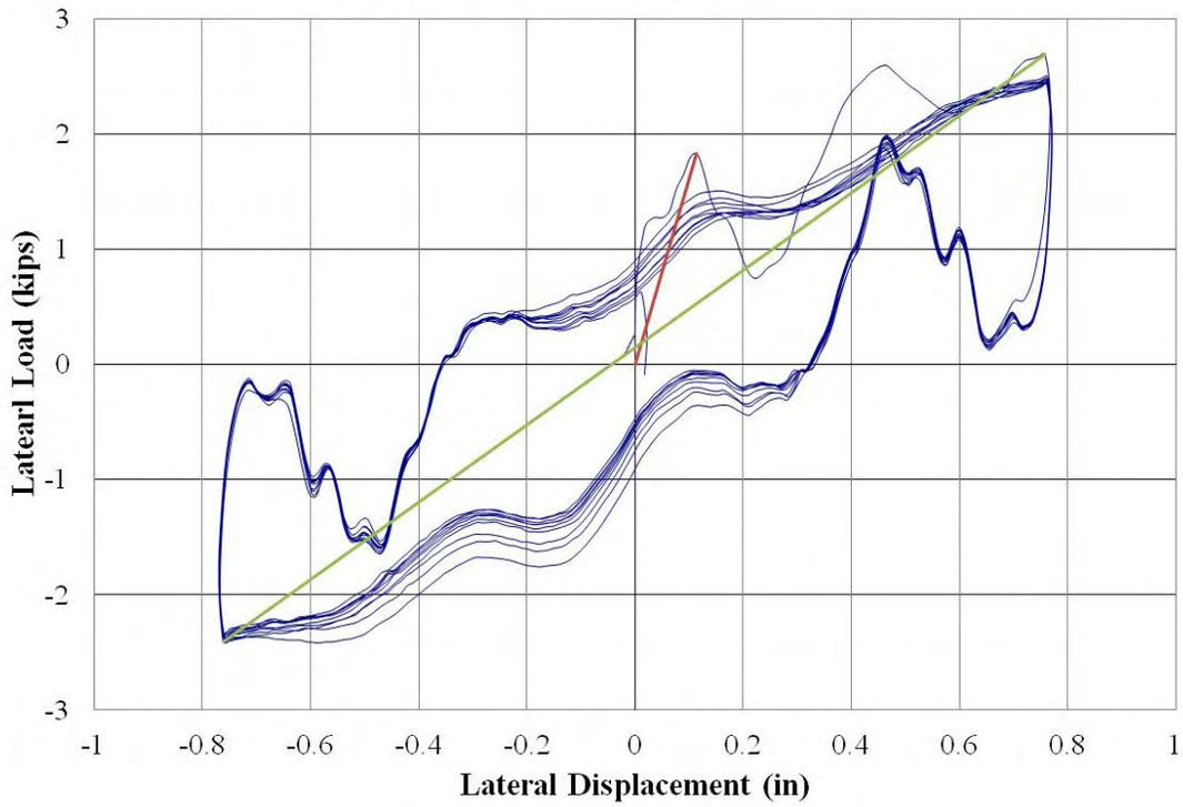
**Figure 68: Retrofit 1 Specimen – 0.75” Cycling**
