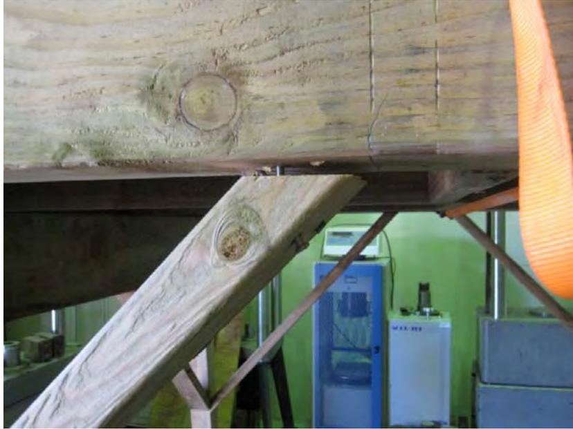
**Figure 32: Control Specimen Nail Pullout Failure at 2x4 Brace**
