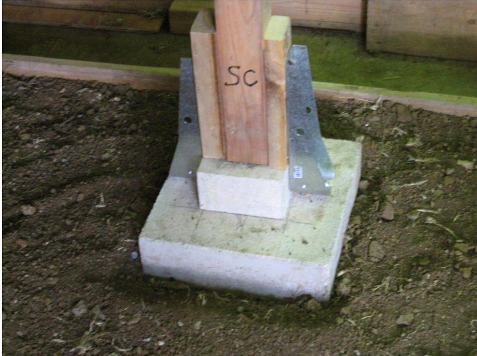
**Figure 6: Typical Partial Retrofit 1 Specimen Tofu Block Foundation**
