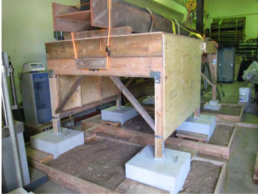
**Figure 17: Specimen 4 with Retrofit Scheme 2 Installed**
