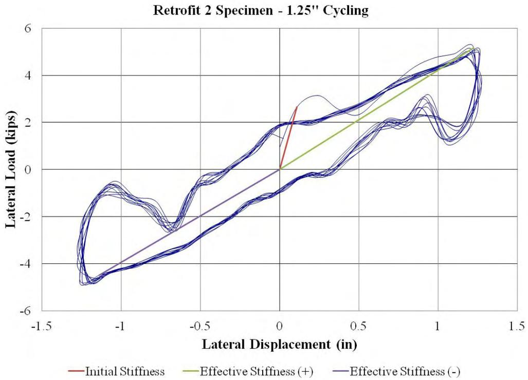
**Figure 83: Retrofit 2 Specimen – 1.25" Cycling**
