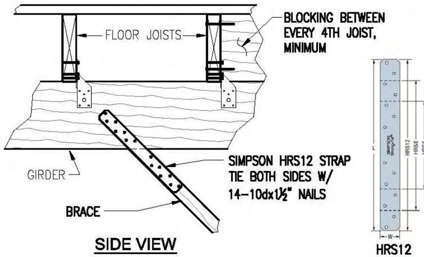
Figure 12: Simpson HRS12 Strap installation
