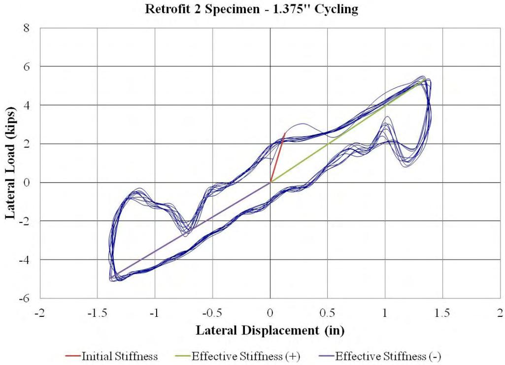
**Figure 84: Retrofit 2 Specimen – 1.375" Cycling**
