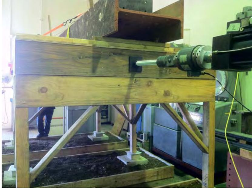
Figure 22: Typical Test Specimen Lateral Loading Set Up
