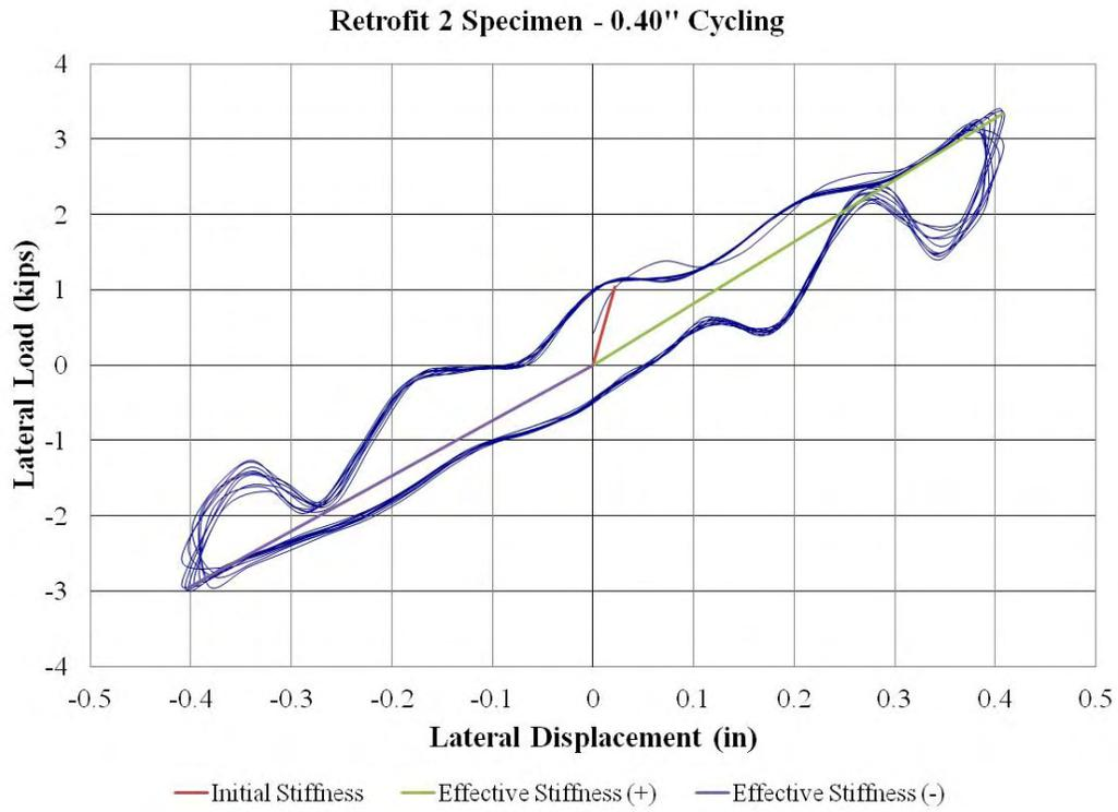
**Figure 76: Retrofit 2 Specimen – 0.40” Cycling**
