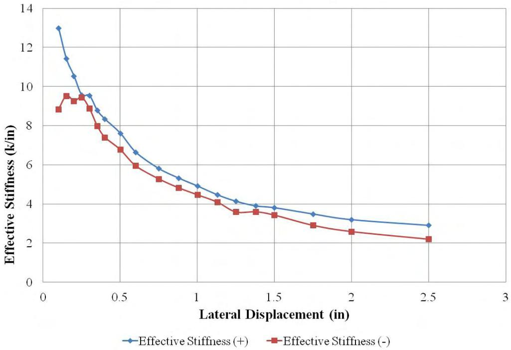
**Figure 49: Retrofit 2 Specimen Effective Stiffness**
