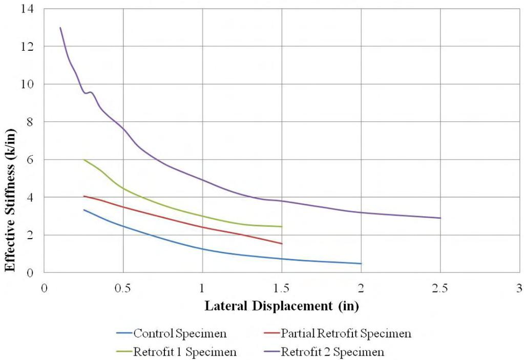
**Figure 54: Specimen Comparison Effective Stiffness (+)**
