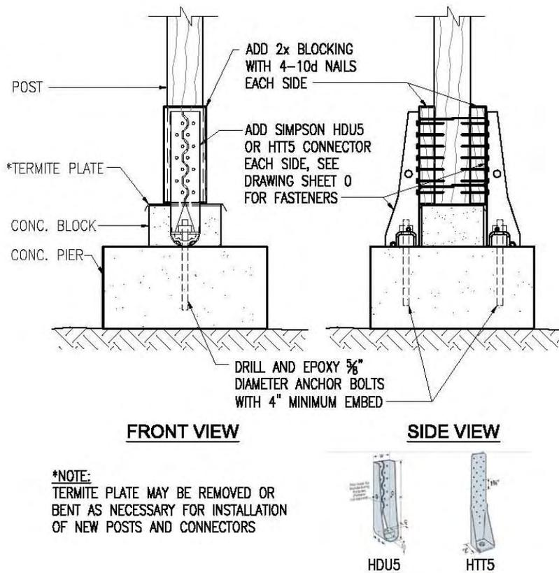
**Figure 7: Simpson HDU Hold-down Connection**
