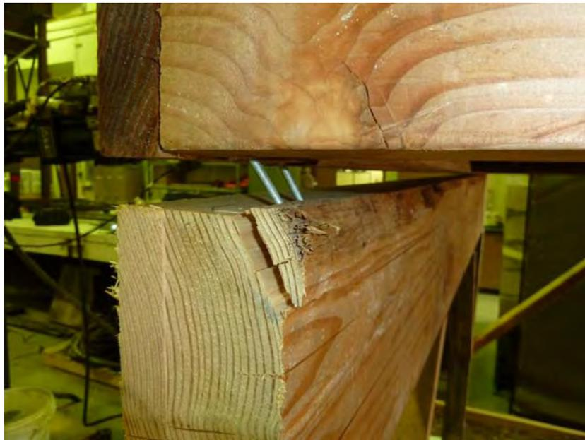
**Figure 33: 4x10 Perimeter Beam to 4x10 Girder Nail Pullout**
