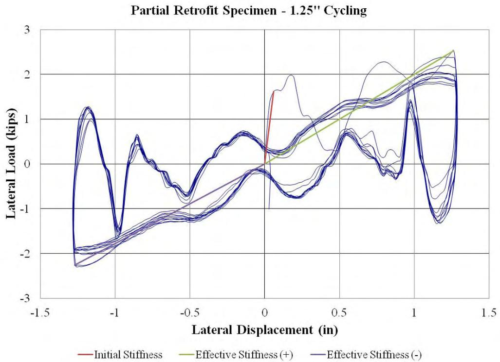
**Figure 35: Partial Retrofit Specimen – 1.25" Cycling**
