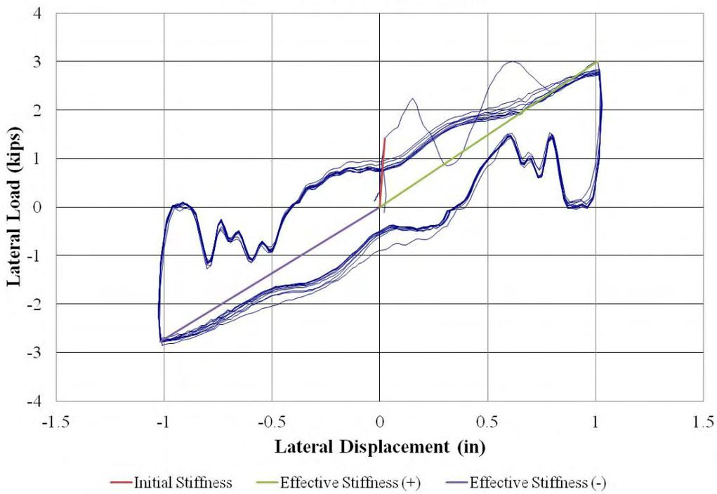
**Figure 69: Retrofit 1 Specimen – 1.0” Cycling**
